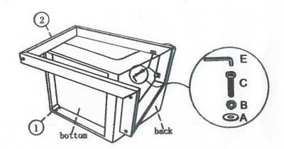
STEP 2 Assemble the holes on front leg and holes under the chair, secure using BOLTS(D) WASHER(B), with ALLEN WRENCH(E), leave Bolts loose by 1/4 turn.
