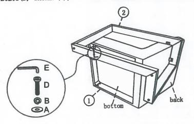
re- tighten the leg bolts after using a period of time
