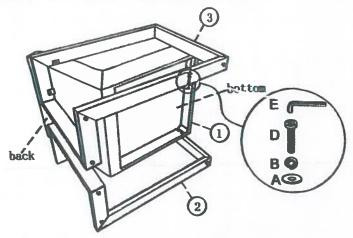
STEP 5 Put the chair on floor to level, then finish tightening all Bolts to 100% turn.
